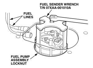
Discard the base gasket between the fuel pump assembly and the fuel tank. Remove the fuel gauge sending unit from the fuel pump assembly.
