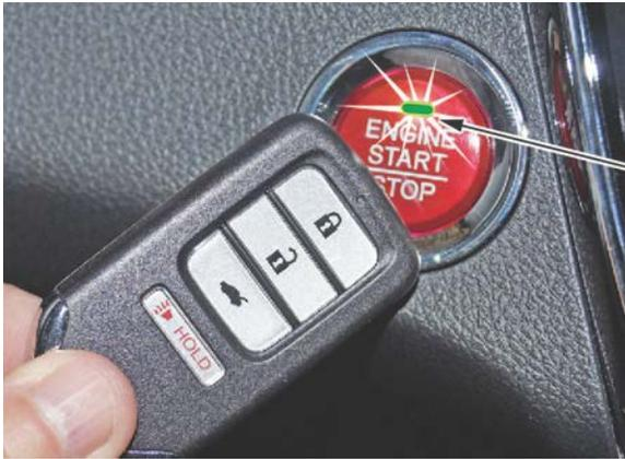
Touch the keyless remote to the blinking ENGINE START/STOP button (blinks for 30 seconds).
