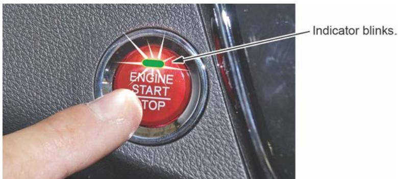
2. When the indicator blinks, touch the keyless remote to the ENGINE START/STOP button.
