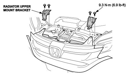
6. Remove the bulkhead upper frame bolts and temporarily insert a spacer on the driver's side of the bulkhead.
