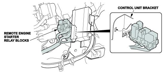
5. Remove the old control unit from the bracket as shown, then unplug the 28P connector and antenna cable from the control unit.
