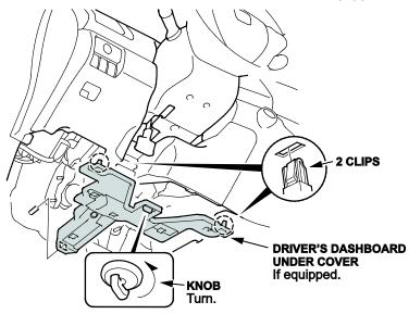
2. Locate the remote engine starter control unit (control unit).
