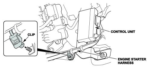
9. Reinstall the remote engine starter relay blocks to the control unit bracket.
