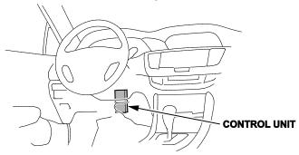
3. Remove the remote engine starter harness clip from the vehicle bolt.
