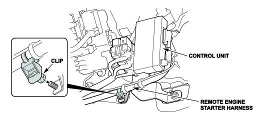
4. Remove the remote engine starter relay blocks from the control unit bracket as shown.
