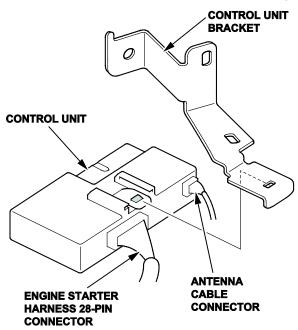
4. Plug the antenna cable connector and the engine starter harness connector into the new control unit.
