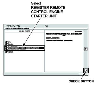
8. The following message will display: **Obtain PCM code (IMMOBILIZER PCM CODE) from the iN. This vehicle's VIN will be required to obtain the password. (USA)** Click on the check button.
