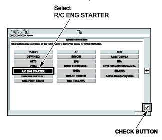
7. Select **REGISTER REMOTE CONTROL ENGINE STARTER UNIT**, then click on the check button.
