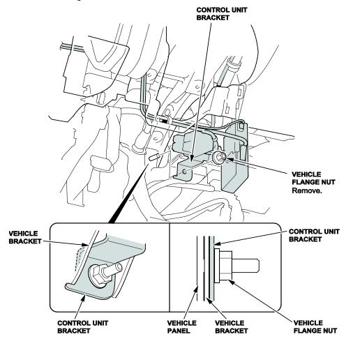
3. Remove the control unit from the bracket. Then, unplug the engine starter connector and antenna cable connector.
