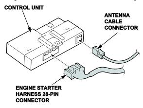
5. Install the new control unit to the control unit bracket.
