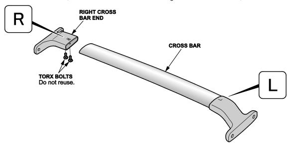
4. Apply 1 square of anti-rattle tape to the end of the right cross bar, as shown.
