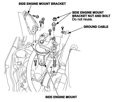
Install the new side engine mount mounting bolts and torque them to 64 N·m (47 lb-ft). Install the side engine mount bracket B using new bolts and torque them to 49 N·m (36 lb-ft), then loosely install the new side engine mount bracket C mounting bolt and nut. Install the ground cable and torque it to 10 N·m (9 lb-ft).
