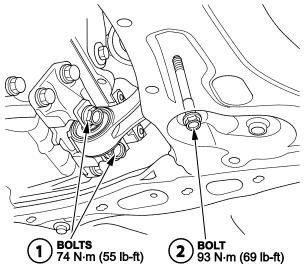
13. Torque the two lower torque rod bolts to 74 N·m (55 lb-ft) and the longer bolt to 93 N·m (69 lb-ft) in the numbered sequence shown.
