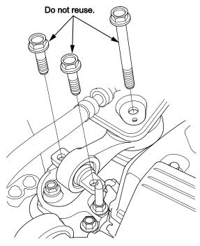
4. Remove the ground cable, the side engine mount bracket, and the side engine mount.
