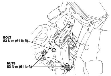
12. Loosen the two lower torque rod bolts.
