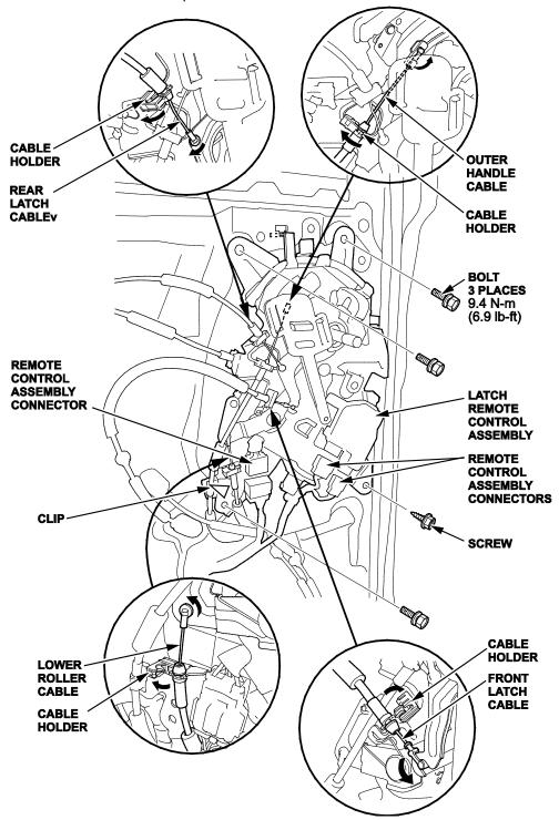
6. Release the cable holder and disconnect the failsafe lever cable from the latch remote control assembly.
