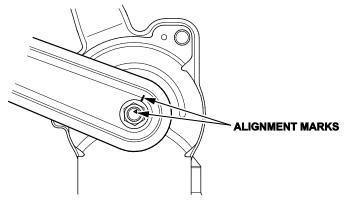
13. Install the new power tailgate arm and torque the bolts to 22 N·m (16 lb-ft) and the nut to 109 N·m (80.41 lb-ft).
