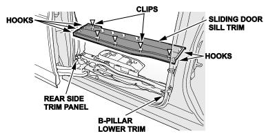
2. Pull out the right sliding door weatherstrip from the trim hooks as needed.
