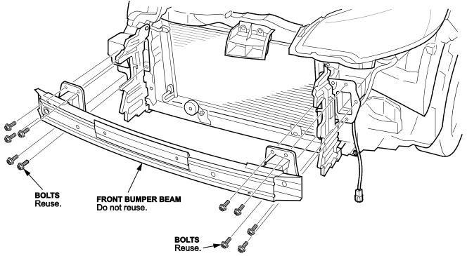
NOTE: Both parts are similar but you can tell the new part from the original part by looking at the weld seams where the bracket connects to the beam as shown.
