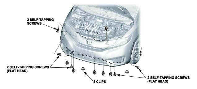
5. Pull out the front bumper at the wheel arch area to release it from the hooks on the side spacer.
