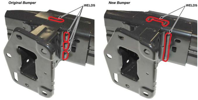
11. Apply a commercially available anti-rust paint like 3M Rust Fighter anti-rust coating (3M P/N 08892) or equivalent to the areas shown, then install the new front bumper beam and torque the bolts to **22 N·m (16 lb-ft)**.
