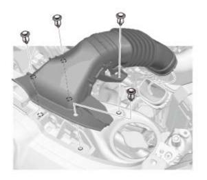
4. Remove front bumper by removing the screws and clips.
