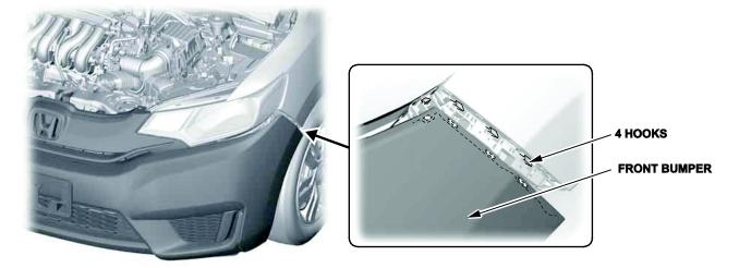
6. With the help of an assistant, gently pull the front bumper away from the side spacer and release the bumper from the hooks on the upper beam, then remove the front bumper.
