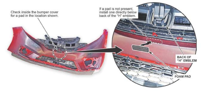
NOTE: There may be two fabric pads located on the front bumper beam. Do not reuse or replace these pads when you replace the bumper beam.
