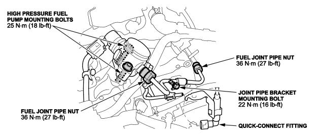
11. Reinstall the parts in reverse order, and then check for any fuel leaks.
