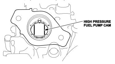
7. Set the No. 1 piston at top dead center (TDC), and then turn the crankshaft 105° counterclockwise. Check the position of the cam that drives the high pressure pump as shown. If the cam position is not correct, continue turning the camshaft until it is.
