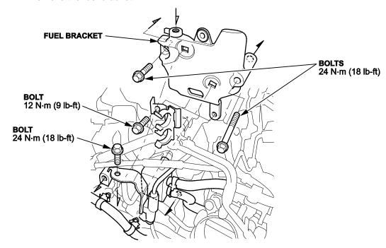
2. Remove the EVAP canister purge valve.
