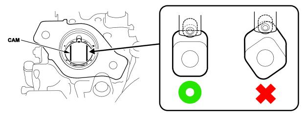
8. Lubricate the cam and roller with clean engine oil, and then install the high pressure fuel pump with the new fuel line clip. Loosely install the bolts.
