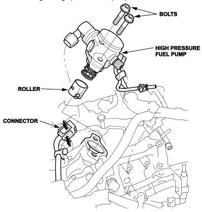
6. Turn the crankshaft and check the high pressure fuel pump cam for any pitting, scoring, or excessive wear. If needed, replace the fuel pump camshaft.
