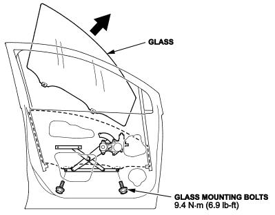
11. Install the new glass through the window slot, then install the glass mounting bolts and torque them to **9.4 N·m** (6.9 lb-ft).
