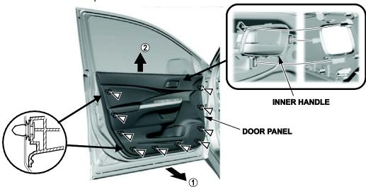
7. Disconnect the connector, and detach the harness clips.
