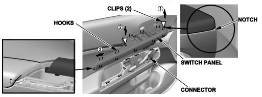
3. Carefully pry out at the upper hook in the inner handle cap, then pull back the inner handle cap to remove it.
