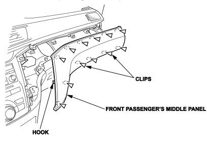
4. From the front passenger's side, pull out the dashboard center panel to release the clips. From the center area, pull out the center panel to release the clips. Then, disconnect the hazard warning switch connector and climate control unit connectors and remove the panel.
