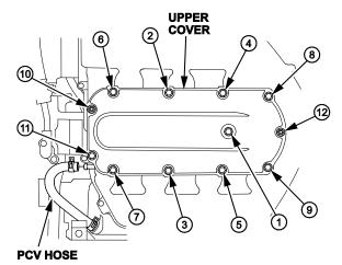
31. Remove the intake manifold bolts and nuts in three steps, then remove the intake manifold.
