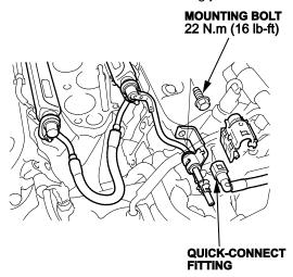
39. Remove the EGR pipe mounting bolts, then remove the EGR pipe.
