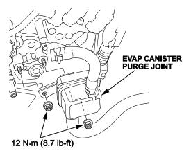
38. Remove the fuel rail connecting joint hose.
