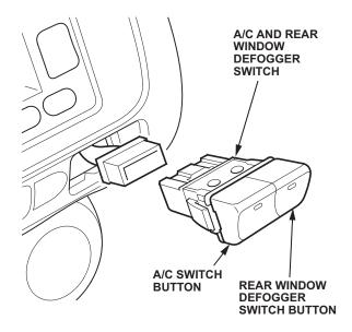
5. Install a new A/C and rear window defogger switch into the center panel by pressing it in from the front of the panel.
