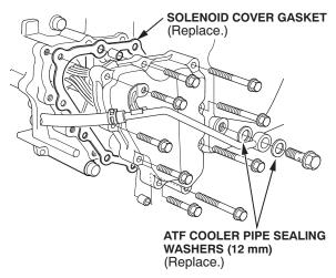
NOTE: Replace the solenoid cover gasket and the ATF cooler pipe sealing washers during installation.
