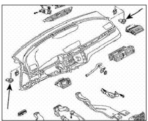
Diagnose the -G150- and/or -G151- temperature sensor (arrows) using normal GFF protocol.
