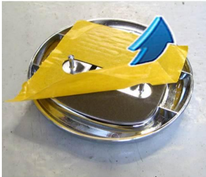
Fig. 6 Remove Adhesive Tape Liner From New Emblem
