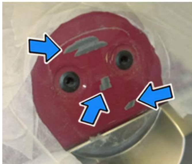
Fig. 2 Remove Residual Adhesive Foam Tape From Liftgate
