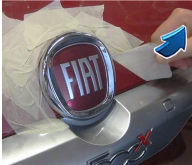
Fig. 9 Remove Protective Masking Material From Liftgate
