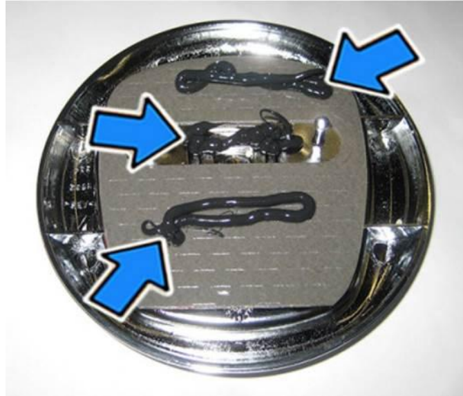
Fig. 7 Apply Adhesive To Emblem Adhesive Tape Surface
