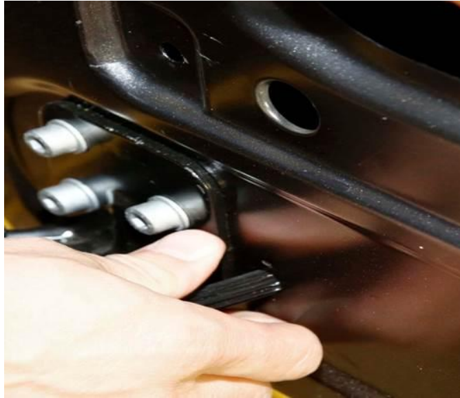
Fig. 19 Routing open latch cable through door
