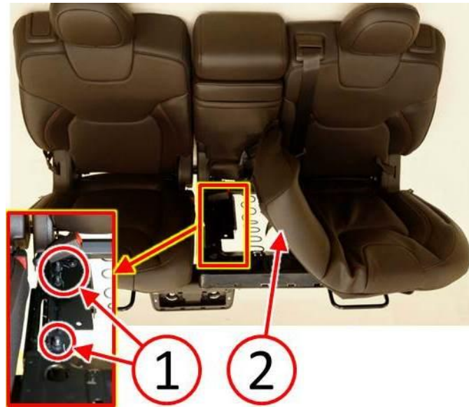
Fig. 7 Access Seat Track Fasteners Under Seat Cushion
