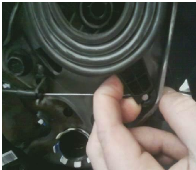
Fig. 4 Hold Cable into Place
