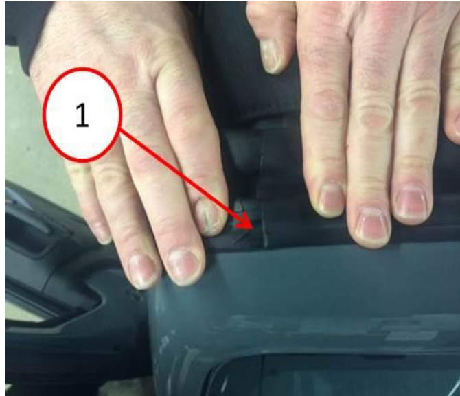
Fig. 1 Header Seal Inspection
