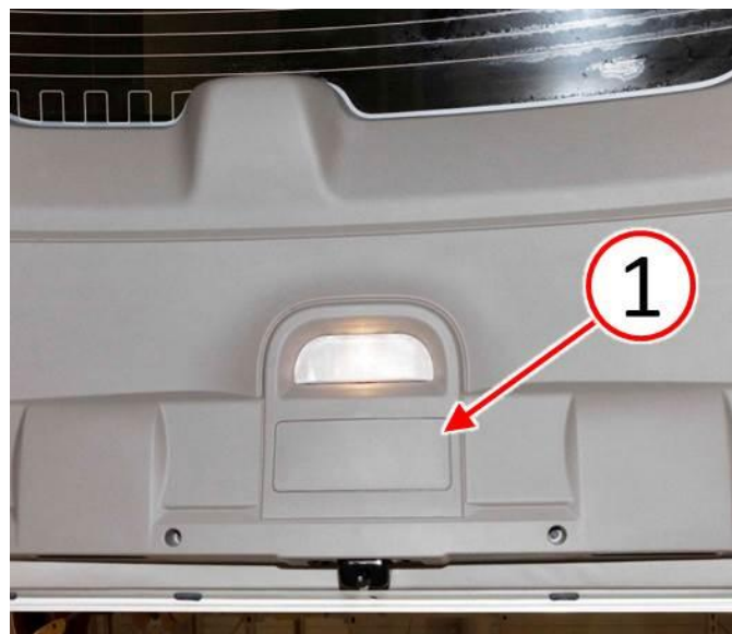
Fig. 9 Install Liftgate Access Panel
