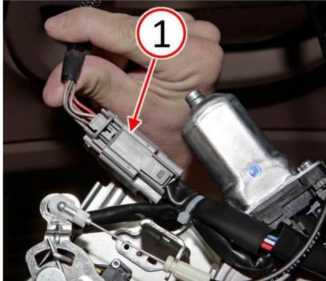
Fig. 4 Disconnect Liftgate latch Electrical Harness
