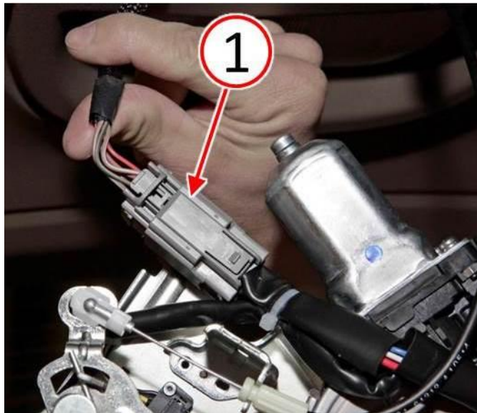
Fig. 7 Connect Liftgate latch Electrical Harness
