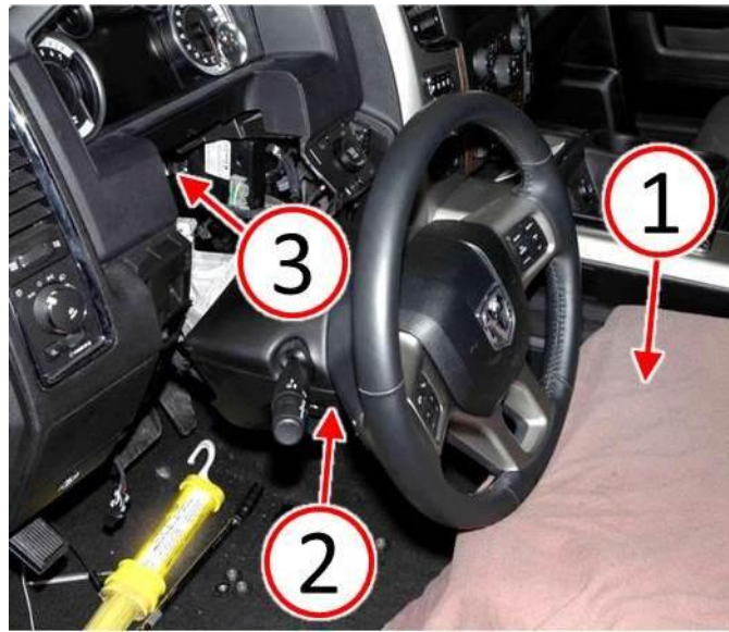
Fig. 5 Protect Seat And Lower Steering Column
