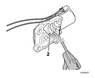
Connect power to solenoid. Solenoid should click. Blow through center hole with compressed air. Air should emerge from outer hole (2).
