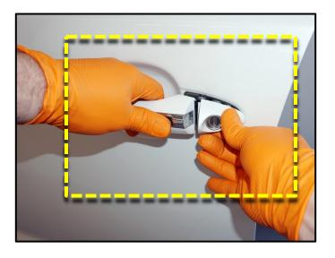
5. Remove the door handle trim cap from the lock cylinder, as shown.
