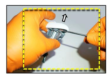
Install the new key-hole trim cap on the original door lock cylinder and reinstall all components by reversing the order or removal. SUBJECT:
