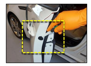
Loosen the key-hole trim cap retaining bolt using a 10mm socket and wrench.
