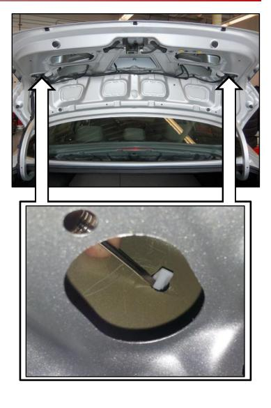
5. If the hooks are not properly engaged, use a flat-head screwdriver to gently spread the clip open, as shown.
