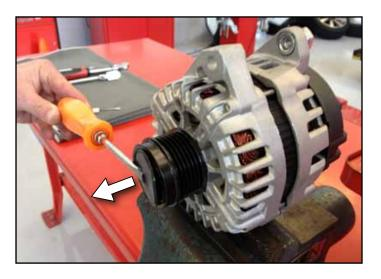
Use the Alternator Pulley Removal /Installer Kit (P/N 09373-27000), to remove the OAD alternator pulley by inserting the removal tool (A) into the pulley splines, as shown.
