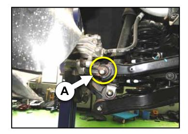
Before installing the rear upper arm to the subframe, support the end of rear lower arm (B) with a transmission jack and raise the jack until the bolt hole of rear upper arm is properly aligned with the subframe (horizontal axis line).
