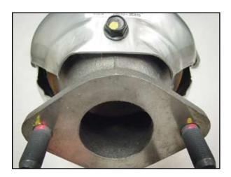
Example of correct heat shield clearance.
