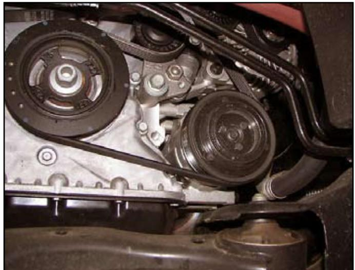
3. Use SST number 09977-29000 to hold the disc + hub assembly.
