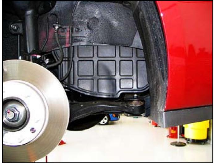
2. Remove the lower engine shield from the wheel well area to expose the A/C compressor / drive belt area, as shown in the photo.
