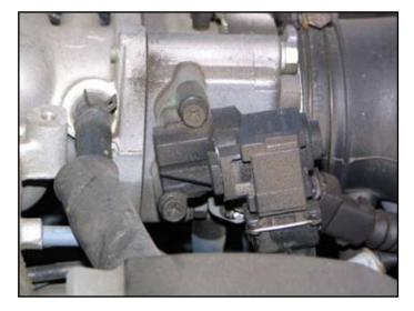
3. Disconnect the throttle position sensor (TPS) connector and remove the two (2) mounting screws.
