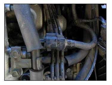
2. Disconnect the idle speed control actuator (ISCA) connector and remove the two retaining bolts. Remove the ISCA and gasket.
