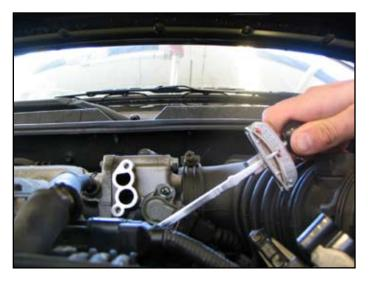
5. Install a new ISCA gasket and re-install the ISCA actuator. Torque the ISCA bolts (6-8 Nm / 52.8~69.6 in-lb), reconnect the ISCA connector. Reconnect the VIS connector and the injector connector if equipped.
