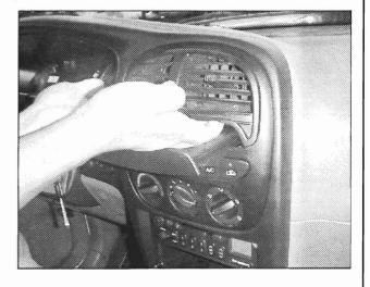
2. Disconnect four (4) HVAC control electrical connectors and remove center panel.
