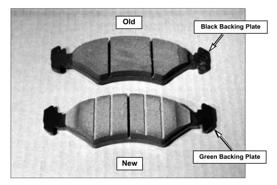
All 2000MY Sephia models are equipped with these improved brake pads. In addition, these new brake pads supercede all previous replacement brake pads for all Sephia models 1994 to present.
