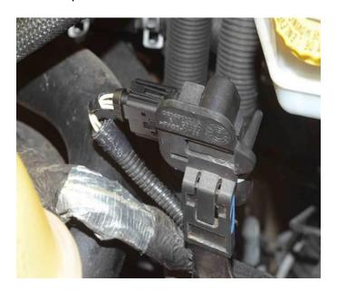
Fig. 4 New Differential Pressure Sensor Reinstalled
