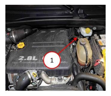
Fig. 1 Differential Pressure Sensor Location - Engine Compartment Location
