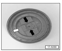
• Position the lower cap so that the molded parallel lines (black arrows) align with the handle of the top portion, and the top piece index mark rests between the parallel lines.
