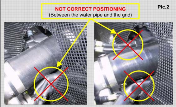
**1.3** If the wiring is not correctly positioned (Pic.2), re-position the wiring <u>under</u> the heat protection grid similar to shown in Pic.1.
