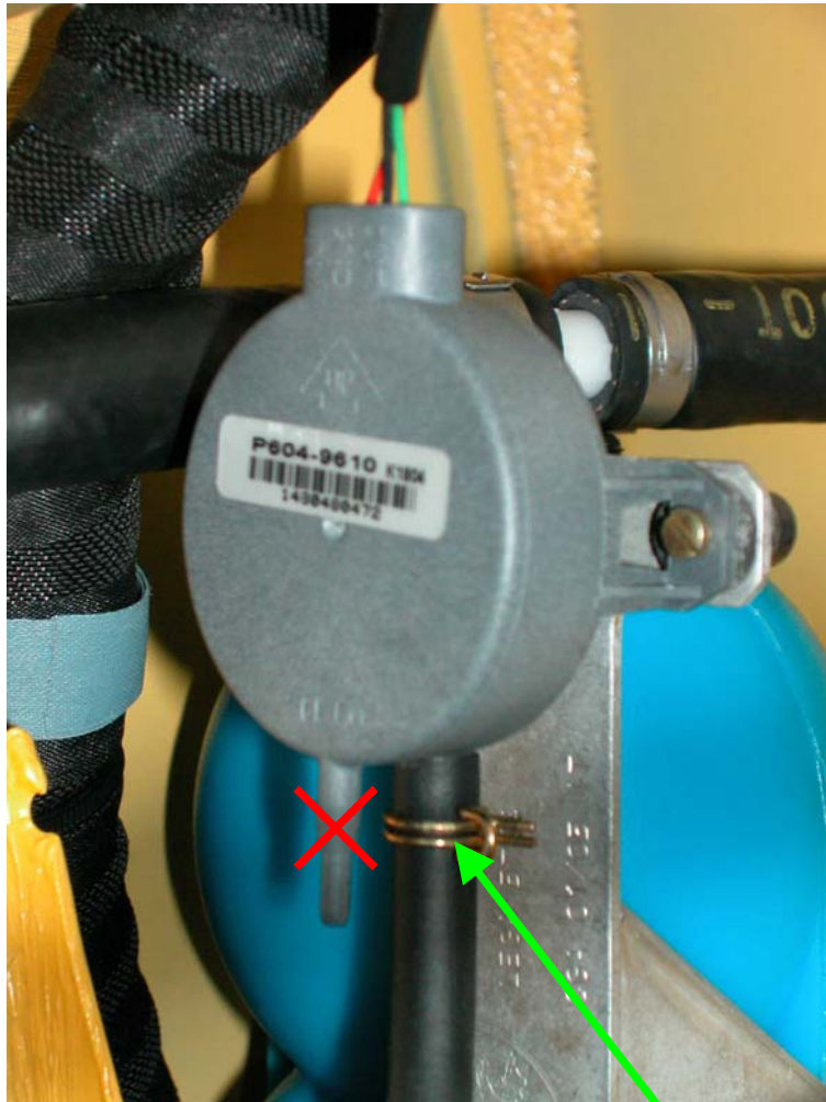
Correct positioning of the pressure sensor inlet pipe.
