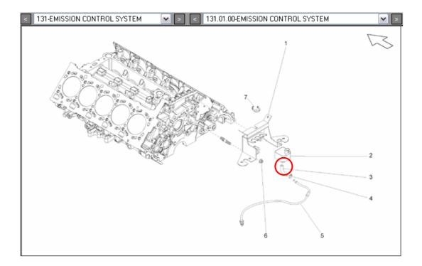
**1.3** Insert the clamps in the pipes where indicated in the picture below.
