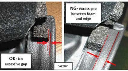
• **EPT Foam Piece #2** is applied to the top front of the door trim panel at the front edge of the inner door glass inner weatherstrip. This piece seals the inside face of the sash and has been pre-cut so it can be properly folded into position as shown in the illustration and photos below.
