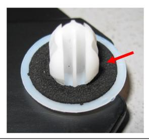
• <u>CAREFULLY</u> release the vapor barrier from the bottom <u>only as much as is required</u> to remove the pad insert, access the window glass and sash retaining bolts and the wiring harness connections the inside door. Tape the vapor barrier to the undisturbed top portion to keep it out of the way. Using a trim clip removal tool, release the retaining clips and remove the plastic pad insert. Use a Philips screwdriver to remove the door speaker.
