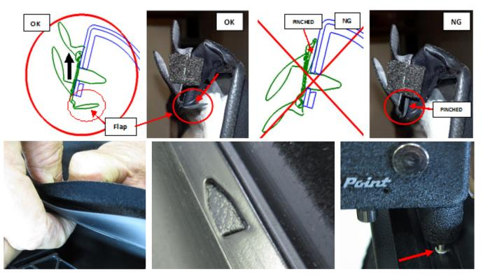
Once all the new claws are bent over and holding the weatherstrip tight against the door panel, install the new retaining rivets using a pop rivet installation tool.
