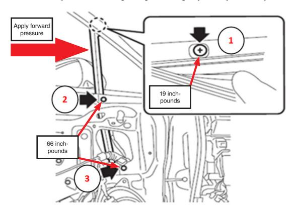
**IMPORTANT**: After the sash hardware has been torqued, make sure the face of the sash is parallel to the top edge of the door as shown in the photo on the right.
