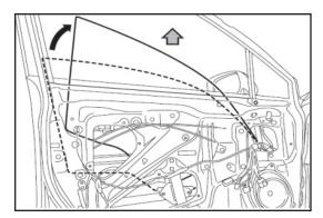
• Remove the #2 Philips screw securing the partition glass sash to the door frame. The screw is accessed by partially removing the outer door seal directly above where the sash meets the door frame. Remove the 2- 10mm hex bolts securing the sash to the inner door structure then remove the sash, partition glass and the run channel as shown in the illustrations below.
