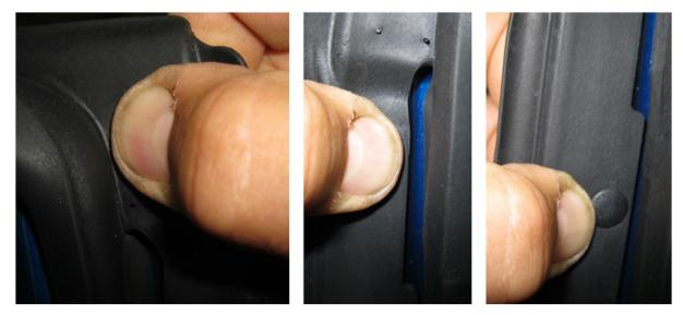
To complete this step, make sure the front of the weatherstrip is properly tucked in behind the chrome outer molding as shown below.
