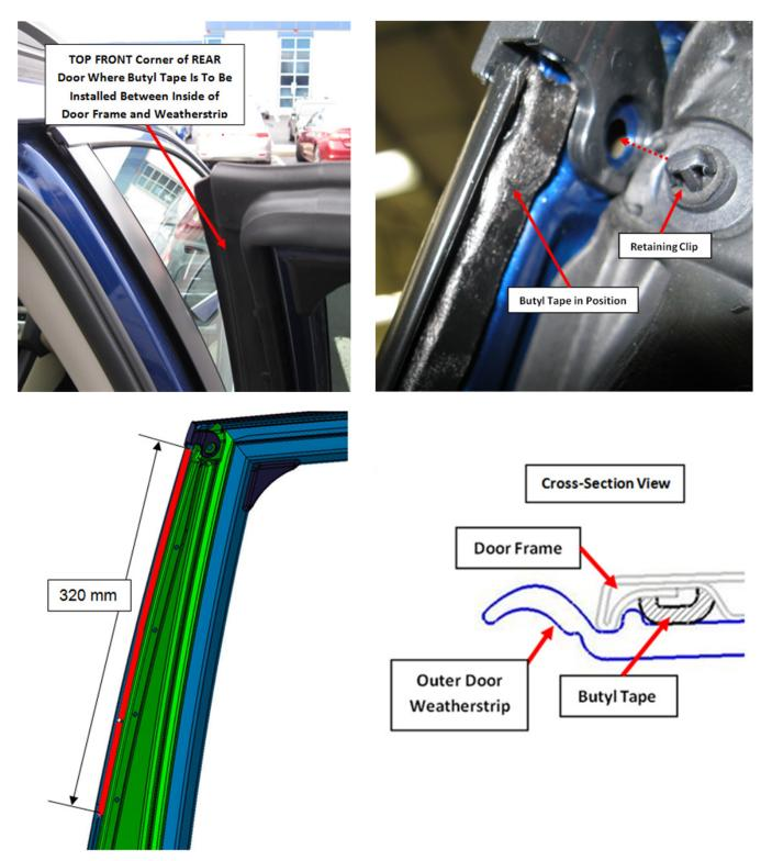
After the butyl tape is applied, refit the weatherstrip and make sure the retaining clip "clips" back into the hole as shown to properly secure and position it. Work the weatherstrip onto the butyl tape with your thumbs making sure it is smooth and any bumps or high spots have been worked out.
