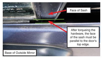
3/8" wide) of 3M .030" thick, Automotive Attachment Tape Part # 06377 (available from any auto body supply jobber) is recommended for this purpose. Leave the adhesive backing in place on the sash-side of the tape until the sash has been reinstalled. Once the sash is in its final position and fasteners properly torqued, pull the deflector out enough to access the sash-side backing of the tape. Peel the backing and press the deflector onto the new sash securing it in place.
