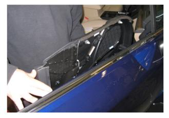
• After disconnecting the wiring harness connections for the power window and door lock switches, armrest pocket lamp, courtesy foot lamp and the speaker, put the trim panel in a safe place to protect it until needed.
