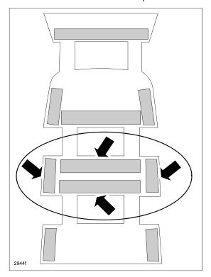
4. Press the two (2) seat warmer bridges (A) into the groove in the pad.
