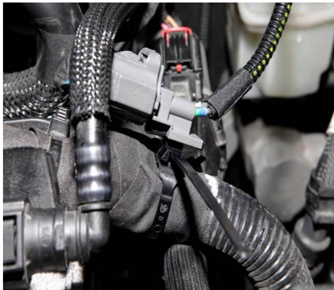
Fig. 5 Location Where Jumper Is Fasten to Harness
