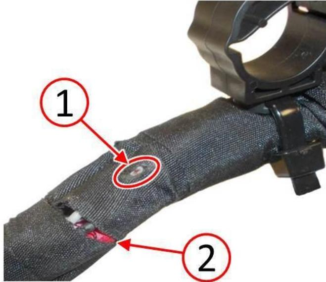
**Fig. 3 Inspect For Harness Damage**
