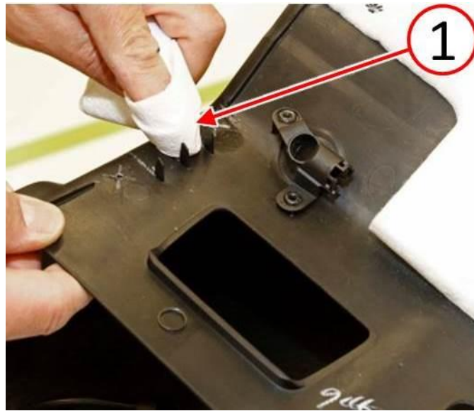
Fig. 20 Clean Alarm Sensor Mounting Surface
