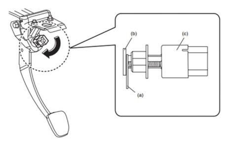
**IMPORTANT:** The stop lamp switch adjustment is **critical** for accurate ABS and VDC control module input along with proper stop lamp operation.
