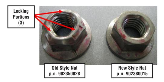
**NOTE:** The nuts are interchangeable between new and old but it is recommended to use all of one style or the other to maintain uniformity. The torque specification is unchanged (14.8 ft. lbs.).
