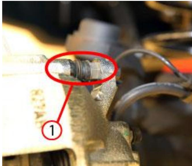
**Fig. 2 Caliper Slide Pin Location**
