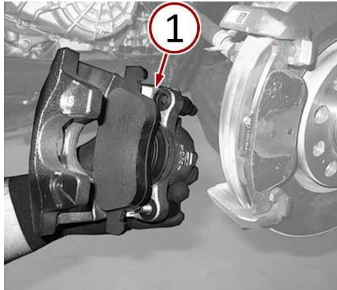
Fig. 8 Install Brake Caliper With Inboard Brake Pad
