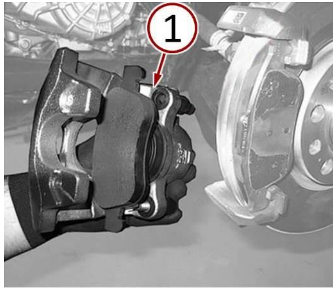
Fig. 2 Remove And Support Brake Caliper
