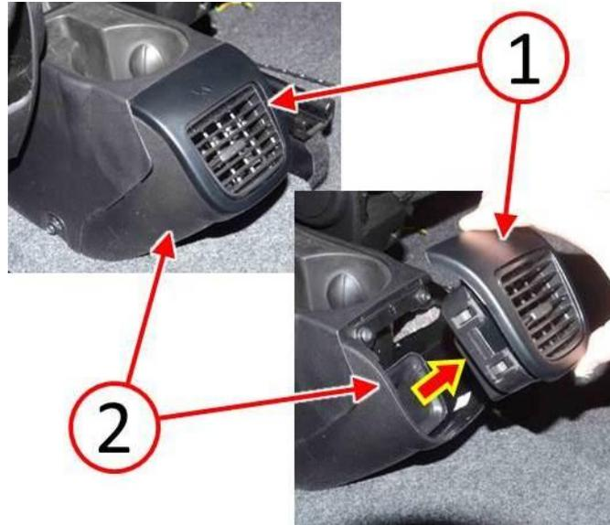
**Fig. 1 Remove Floor Console Air Outlet**
